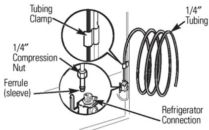
Fasten the tubing into the tubing Clamp attached to the back of the refrigerator.
